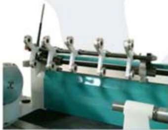
Wire Guide Bars for Winding Multiple Coils
